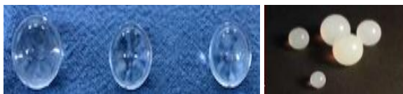
Fig. 2 (a) Acrylic non porous spheres and (b) Silicone spheres
